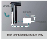
High air intake reduces dust entry
