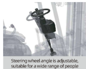
Steering wheel angle is adjustable, suitable for a wide range of people
