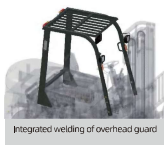
Integrated welding of overhead guard
